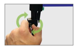
**Step 6:** Twist the butterfly screw to secure the locking mechanism.
