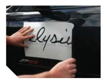
Apply magnetic sheet directly to the vehicle. Do not pull magnet to reposition
