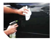
The surface of the vehicle & surface of the magnet must be clean and dry.
