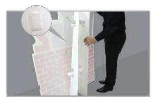
**Step 5:** To attach the Strut to your Standee, simply hold both objects upright and align the hook and loop velcro to the allocated sections. It is important to align the base of your Standee and Strut so they balance upright.
