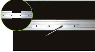
**Step 4:** \*If your frame is over 1500mm, slide the splice connectors into the grooves. Butt spliced pieces of the frame together and use an allen key to tighten set screws on splice connectors.
