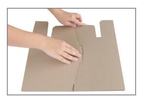
**Step 12:** Tuck the corner flap on one side of the header board into the cutout slot on the other side and press it down until it is flat.
