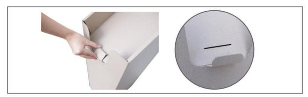
**Step 10:** If you are inserting the shelf of the open front dump bin, make sure that you pull the small tab on the front of the dump bin out and then insert the side of the shelf with a slot cut out in the front side of the dump bin. Slide the shelf into the dump bin as shown in the previous step and insert the tab in front of the dump bin into the slot on the shelf.
